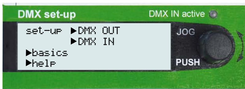
First level - knob EFFECT in position "DMX set-up"
